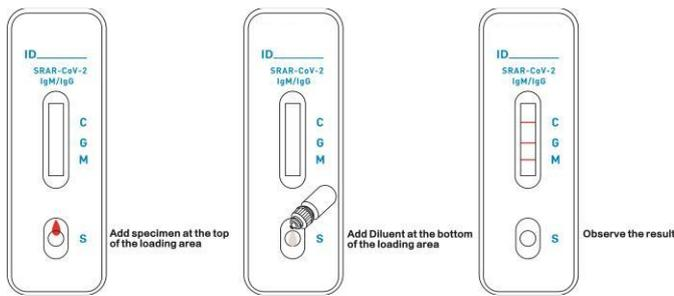
Figure 1 Schematic diagram of card type test procedure
