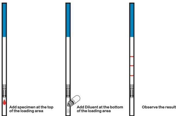
Figure 2 Schematic diagram of strip type test procedure
